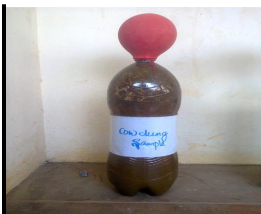
Figure: 1- Biogas Production within Cow Dung Sample on 2 nd Day
